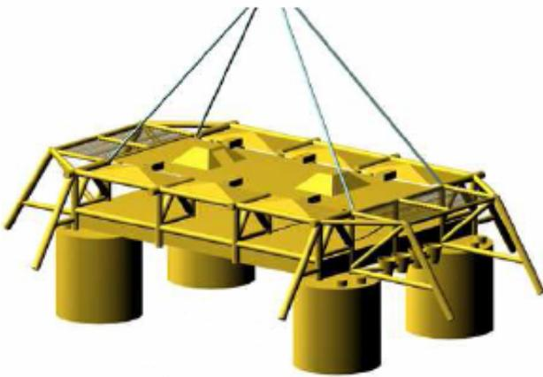
Figure 4. A subsea template
