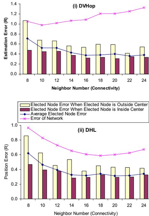
Figure 5. Error of elected anchor compared with all other nodes for (i) DV-Hop and (ii) DHL
