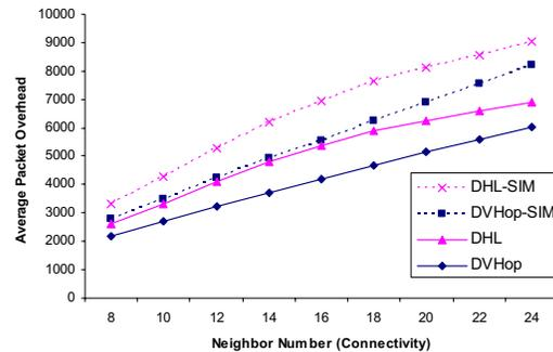
Figure 7. Average packet overhead with varying connectivity
