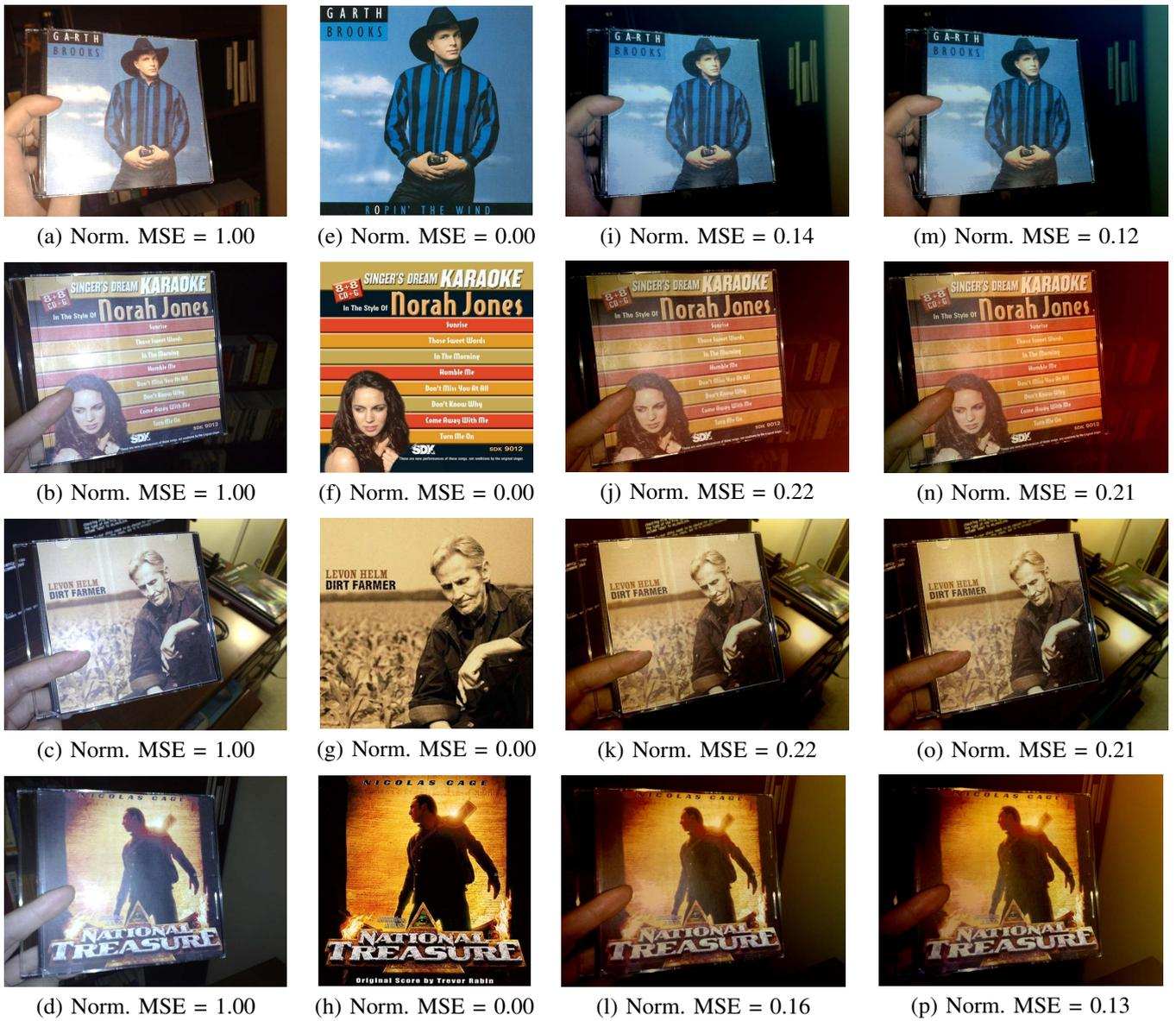
Fig. 5. (a-d) Unprocessed query images. (e-h) Database images. (i-l) Restoration with linear model. (m-p) Restoration with piecewise linear model.
