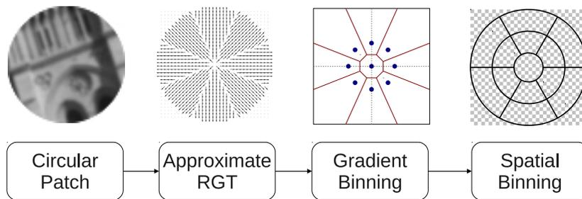
Figure 1. Descriptor computation pipeline. We start with a circular image patch and then compute the Approximate Radial Gradient Transform (ARGT) on the patch. Each gradient is then quantized before being placed in the appropriate spatial bin.
