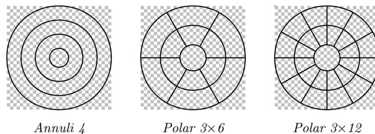
Figure 2. Cell configurations for spatial binning. More cells increases distinctiveness, while larger cells increases robustness to scale and offset errors.
