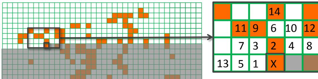
Figure 3. The location histogram map is encoded in a raster scan order. The darker blocks indicate uncoded blocks while the orange blocks indicate non-empty blocks. For each block, nearby previously encoded blocks are used as context as shown in the right.
