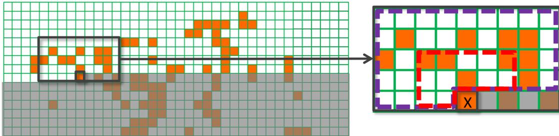
Figure 4. For each block, nearby previously encoded blocks are used to generate the context. In the close up view, the red and purple dashed lines encloses the neighboring blocks used to generate the sum-based context for a range of 2 and 4, respectively.
